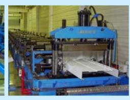
The lines can be equipped with flying scissors that provides the production capacity of 60 m/ min, i.e. 20 sheets (4 m length) per minute.
