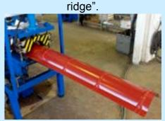
Rollforming lines LPS series are designed for manufacturing of siding-panels («ship board», «L-beam», «log», «beacon», «angle», etc.), decorative profiles, profiles for fixing plasterboard plates and other special profiles.
