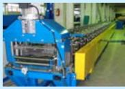
Rollforming Lines LPA series are intended for manufacturing of various reinforcing profiles (with perforations, knurling or without).
