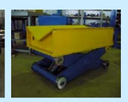
Decoiler RP series (driving, with manual coil clamping)
