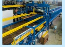
Rollforming Lines LPEK series are intended for manufacturing of roof Rollforming Lines LPKM series elements such as "wind board", "angle", "ridge", "cornice plank" etc.
