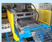
Rollforming lines LPP series are Rollforming lines LPKP series Rollforming lines LPSHR designed for manufacturing of panels are designed for manufacturing series are designed for of different configurations (racking of profiles for fixing front panels, manufacturing of profile systems, linear and other front panels).
