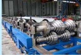
Roll forming Lines (mono) LPRF series are designed for manufacturing of only one type of corrugated profile (corrugated board, cassette profile, panels of prefabricated buildings, etc.) with a width of up to 1600 mm, thickness up to 3 mm, profile depth up to 250 mm. Maximum profiling speed - 40 m/min.
