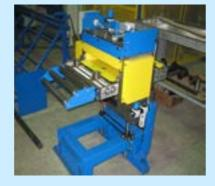
**Perforating machines** are designed for making spherical deformation plots on the original strip by means of rotation in order to increase its rigidity.
