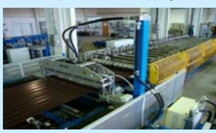
**Conveyors and stackers** are designed for stacking sheets in a pack and issuing them along and across the axis of profiling.
